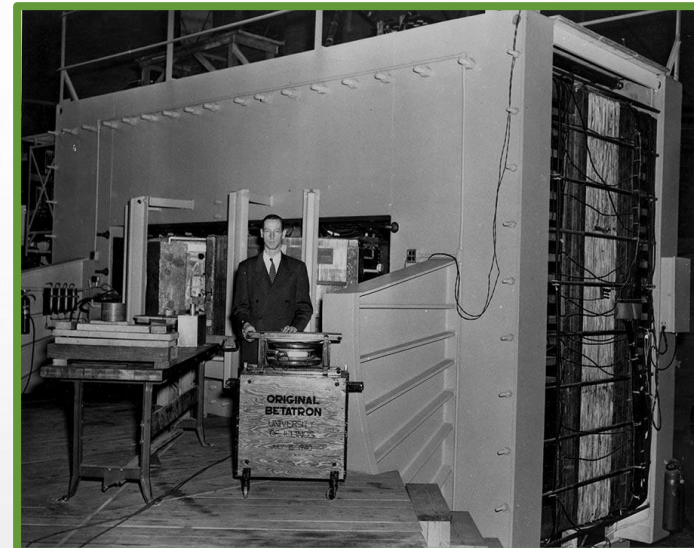
Prof. Donald W. Kerst with the world's first betatron, built at the University of Illinois in 1940
